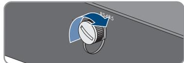
5. Unscrew the swivel nut from the threaded sleeve for the network cable.
